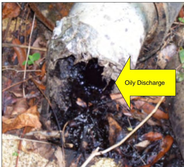
“Close Up” photo of discharge of oily substance from pipe. Provides good detail of the nature of the illicit discharge.
